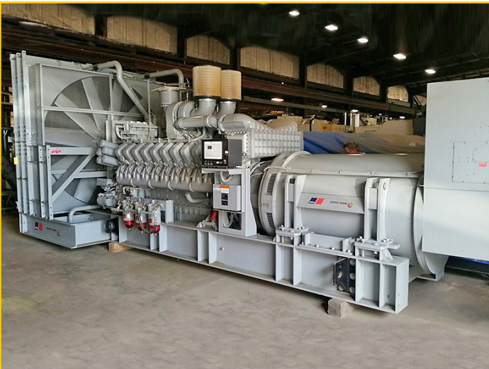
#5363 MTU Diesel 3000 kW RXC6DT2, 480V, 0 Hrs, New Surplus 2007, EPA Tier 2
