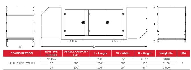
\* All measurements are approximate and for estimation purposes only. Weights are without fuel tank. Sound levels measured at 23ft (7m) and does not account for ambient site conditions.
