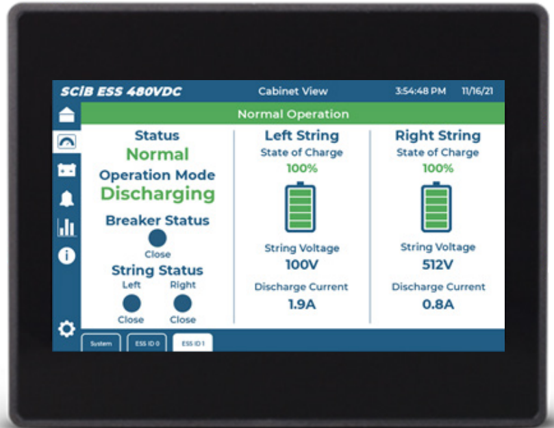
(Fig.1) Cabinet String Level View
