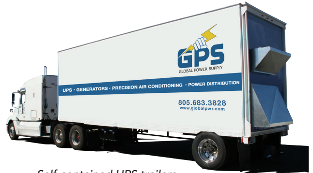
Self-contained UPS trailers up to 1,000 kVA
